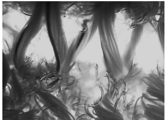
Figure 4.—Detail of the fabric with copper and zinc threads covered with polyamide.
