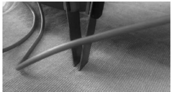
Figure 5.—Measuring the microcurrent with measuring electrodes on the knitted fabric.
